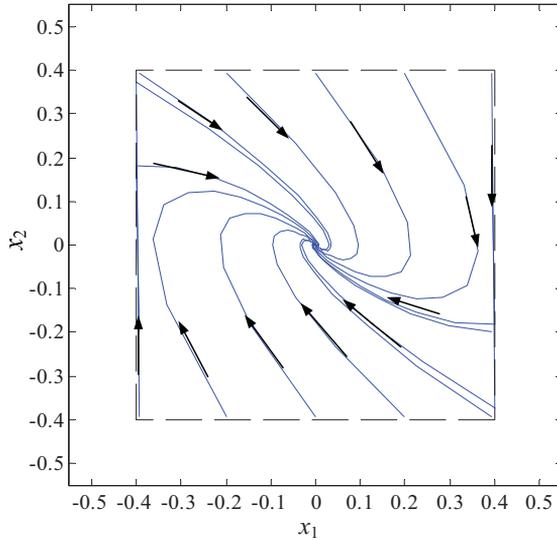
Fig. 3. Phase portrait of the system (18)-(19) using the NMPC.
