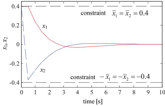
Fig. 6.  $x_1(t)$  and  $x_2(t)$  of system (18)-(19) using the NMPC control law:  $x_1(t)$  and  $x_2(t)$  converge to zero in 10 s while the constraints are not violated.
