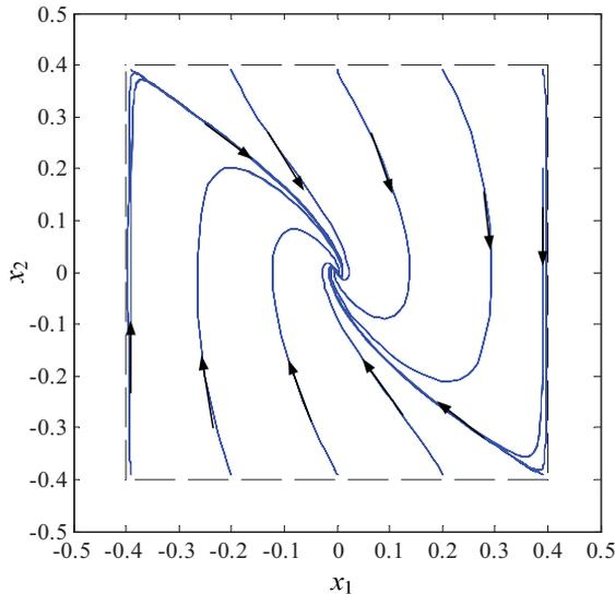
Fig. 1. Phase portrait of the system (18)-(19) using control law derived from the barrier function as the Lyapunov function.
