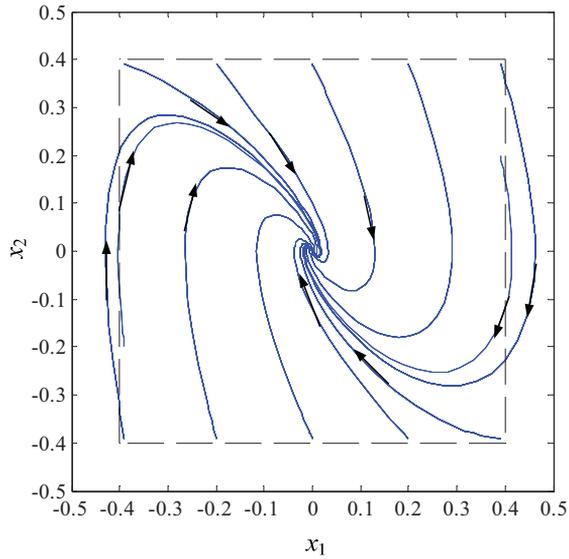
Fig. 2. Phase portrait of the system (18)-(19) using using the control law derived from the quadratic Lyapunov function.
