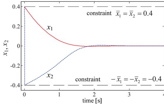
Fig. 4.  $x_1(t)$  and  $x_2(t)$  of system (18)-(19) using barrier-function-based control law:  $x_1(t)$  and  $x_2(t)$  converge to zero in 3 s while the constraints are not violated.
