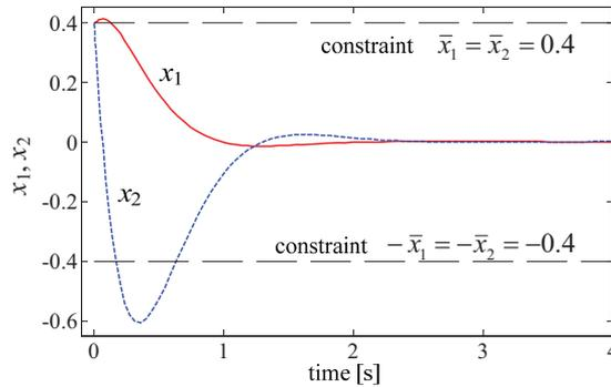
Fig. 5.  $x_1(t)$  and  $x_2(t)$  of system (18)-(19) using quadratic-function-based control law:  $x_1(t)$  and  $x_2(t)$  converge to zero in 3 s, but both violate the constraints.
