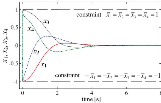
Fig. 8.  $x_i(t)$ ,  $i = 1-4$ , of the system (30)-(31) with barrier-function-based control law.
